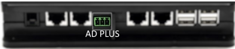
Figure 9A - Connector position in the AD plus and DConnect box, e.g. can-bus straight cable connection, connector name DConnect box for connection with AD plus
